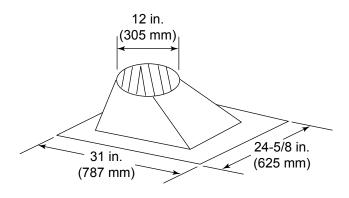
**RF371 Roof Flashing**
